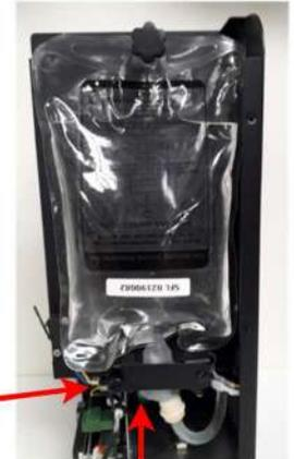
Ensure the consumable neck is held correctly and the fluid micro switch is closed
