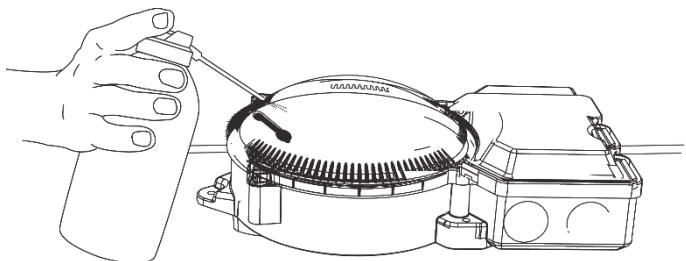
Check the airflow around the detector with a suitable smoke detector tester. Move the "test hole plug" to the side and briefly release a spray of aerosol smoke. Check the detector goes into alarm, i.e. the red alarm LEDs are activated. Also inspect the appropriate fire control panel indicators.
