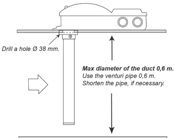
For ducts with a  $\varnothing$  of less than 0,6 m use the 0,6 m pipe, standard.
