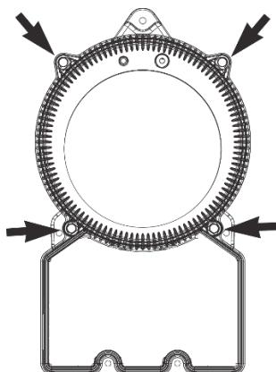
The smoke detector or sensor is mounted on a base which is fixed and wired to the SDP-3. The mounting base needs to be mounted on the centreline of the unit, using the provided fixing holes.
