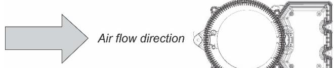
*The SDP-3 smoke detector must be installed pointing towards the air flow direction.*
