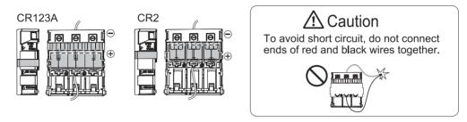
3 Connect the alarm cable to the transmitter and close the cover.
