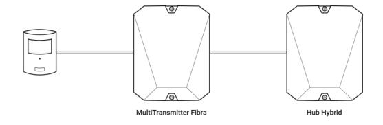
MultiTransmitter Fibra can be used for integration of panic and medical alert buttons, indoor and outdoor motion detectors, as well as opening, vibration, breaking, gas, fire detectors, etc.
