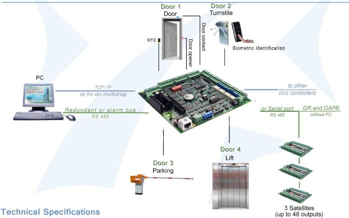
Board dimension: 175 x 160 x 20 or 32 mm Operating temperature: 0° C to +55° C Storage temperature: -10° to +65° C Operational humidity: 10 to 95% RH
